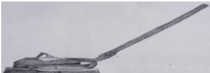
Fig. 4: Cutter (Mkpachi): A Tool used to cut metal Drawn by Nzoiwu Azuka 2017
